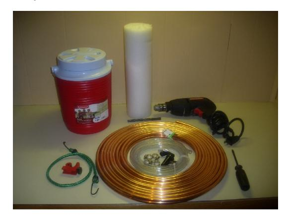
Once you have the above equipment, the time to build the mini-chill is less than one hour. First, you find out whether the item you plan to wrap the tubing around fits within your cooler with at least 1 inch to spare around it. This will give you space to wrap the coil around and also allow for water and ice circulation to keep the device chilled. We are going to create a
